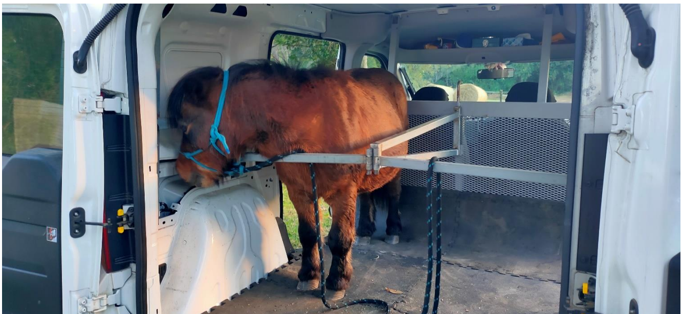
Picture: the very large and the very small equines simply do not fit in standard, commercial horse transport. This vehicle has been customised to safely transport two (2) miniature horses, with rear facing bays, a reinforced cargo barrier, and additional ventilation.
